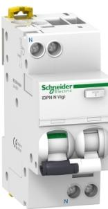
Residual current breaker with overcur. prot. (RCBO), Acti9 iDPN N Vigi, 1P+N, 25A, C curve, 6000A, A-SI type, 30mA
